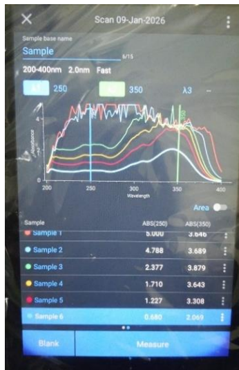
Figure 6. UV-Vis Spectrum Results of Black Pepper Crystals (Bottom Graph)
