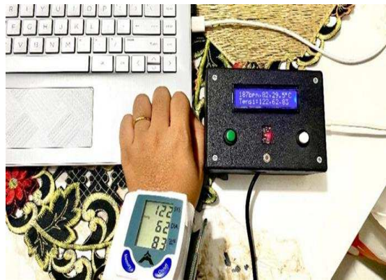
Gambar 5. Prototype Alat Monitoring Tanda Vital Berbasis IoT
