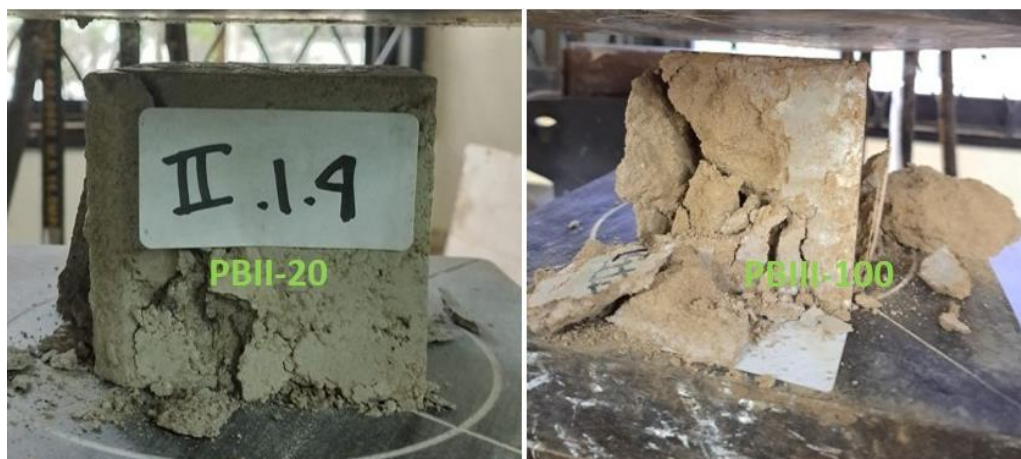
Figure 4. Failed cubic specimens under compression.
