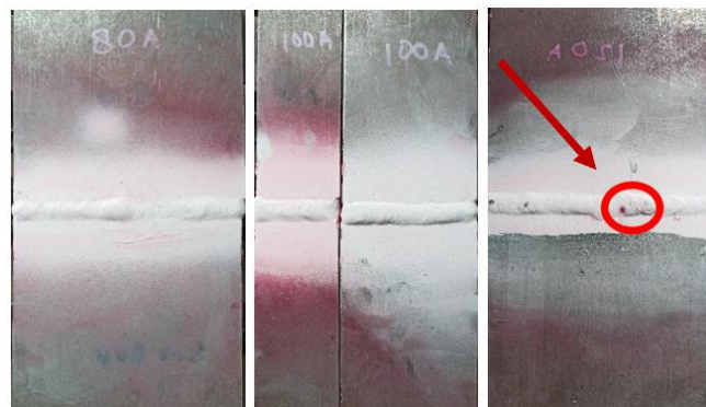
Fig. 6. Penetrant Test Results
