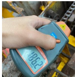
Gambar 5. Validasi Sensor RPM
