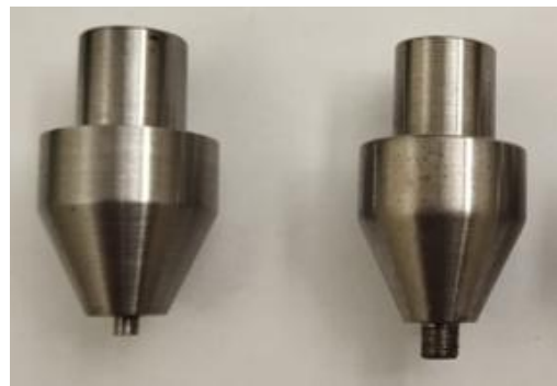
Gambar 10 Alat gesek FSW, (a) pin silinder, (b) pin silinder berulir
