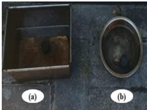
Gambar 7 Proses Pendinginan Material, (a) Air Tawar, (b) Air Garam
