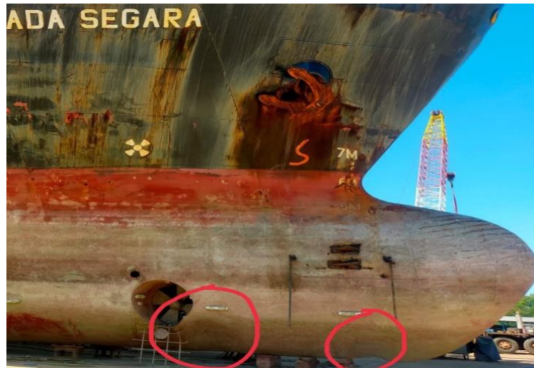
Picture 7. Dented Section in Bulbous Bow Source: Personal Documentation (2022)
