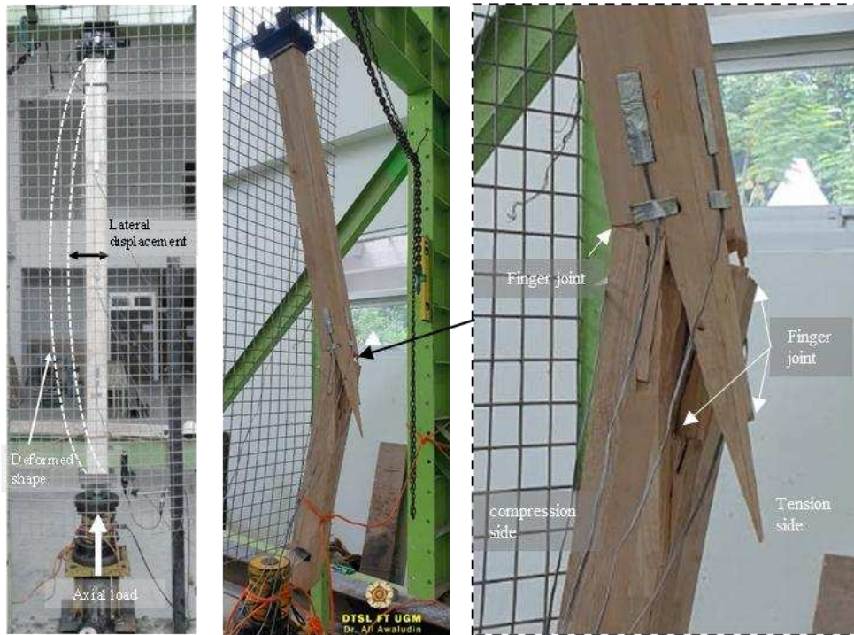
Figure 5. The Buckling Failure of the Specimen
