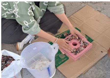
Figure 2. Hand Lay Up or Compression Molding Technique (Source: Primary Data, 2025)
