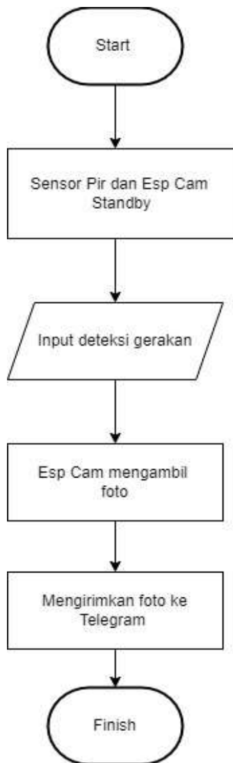
Gambar 2. Flowchart sensor pir + ESP-cam
