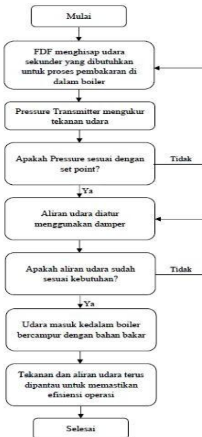
Gambar 4. Flowchart Cara Kerja Forced Draft Fan (FDF)
