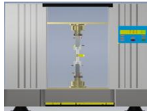
Figure 4. The Crack testing machine with COM-TEN Brand 95T Series 5K.
