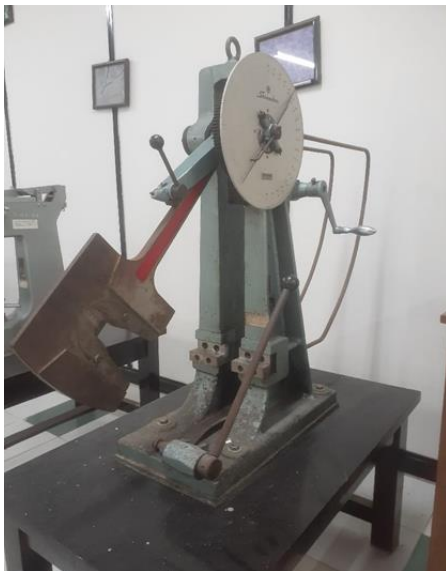
Gambar 1 Uji impact Charpy
