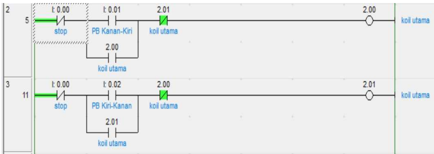
Figure 9. The third push button is given a high condition to stop the operation of the three-phase induction motor
