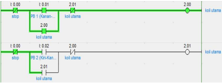
Figure 6. Simulation of the first pushbutton given high condition
