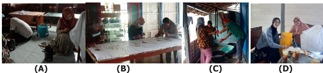
Figure 4. (A) The batik canting process, (B) Coloring process, (C) Fixation and wax removal process, (D) Researcher with Mrs LS (Samin Sambongrejo Batik Maker)
