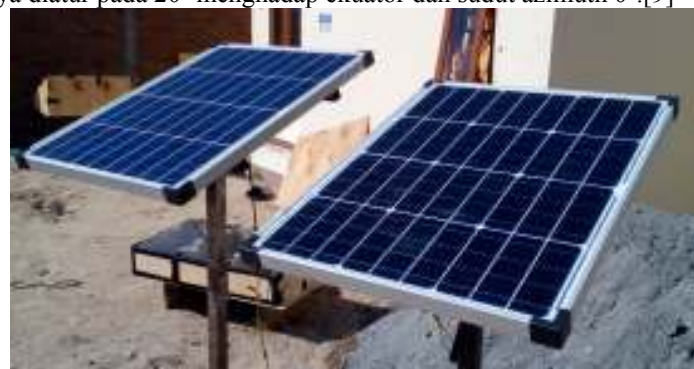
Gambar 2. Set up panel surya polycrystalline dan monocrystalline
