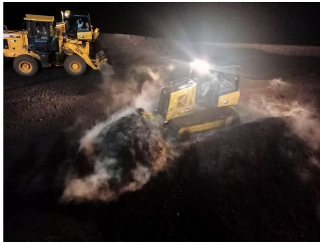
Figure 2. The process of cooling down cargo using a bulldozer Source: researcher documentation
