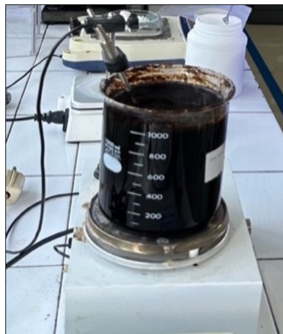
Figure 3. Delignification process on banana peel CMC samples
