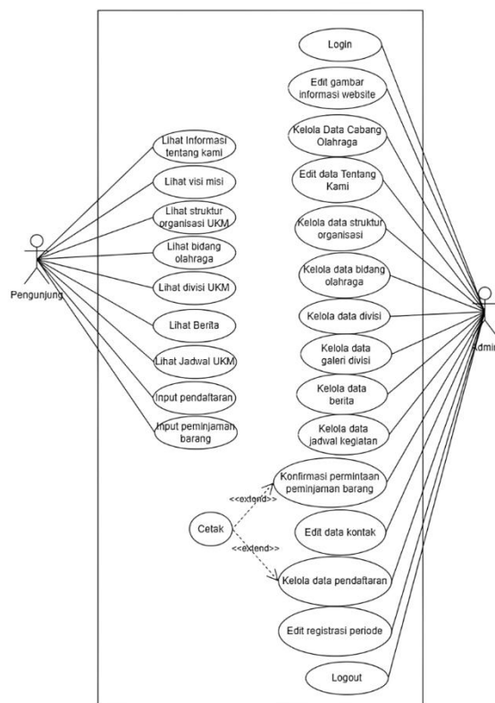
Gambar 3. Use Case Diagram Sistem
