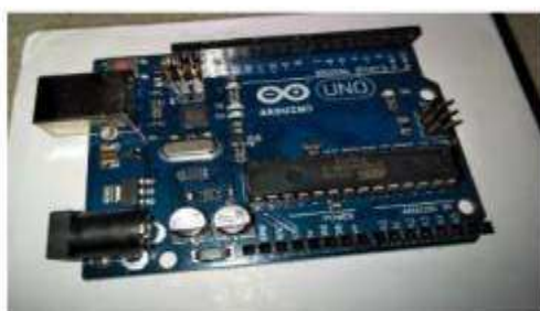
Figure 2. Physical form of Arduino Uno Source : (Banzi & Edition, 2011)
