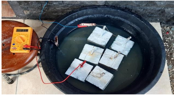
Gambar 6. Proses Pemberian Initial Corrosion
