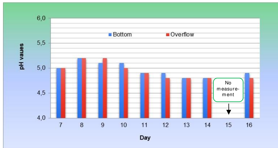
Figure 5. The pH value at the bottom of reactor and at the overflow
