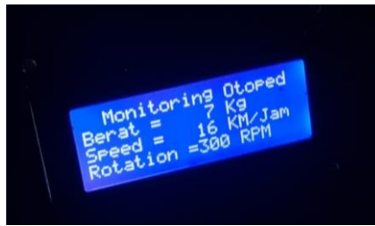
Gambar 10. Tampilan LCD Saat Sistem Monitoring Otored Bekerja
