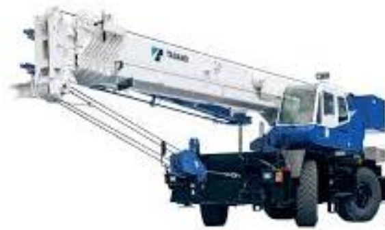
Gambar 3. Mobile Crane Tadano GR-500EXL.
