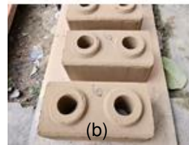
Figure 1. Sample Interlock brick specimens (a) 8%, (b) 9%, and (c) 10%
