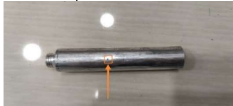
Figure 7. Leak in the tube
