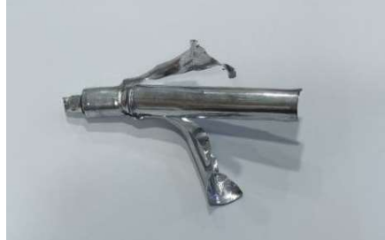
Figure 6. Extreme Damage to the tube
