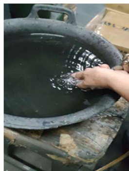
Figure 5. Tube Leak Testing
