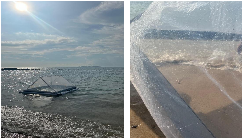
Gambar 2. Uji coba Solar Still di Laut
