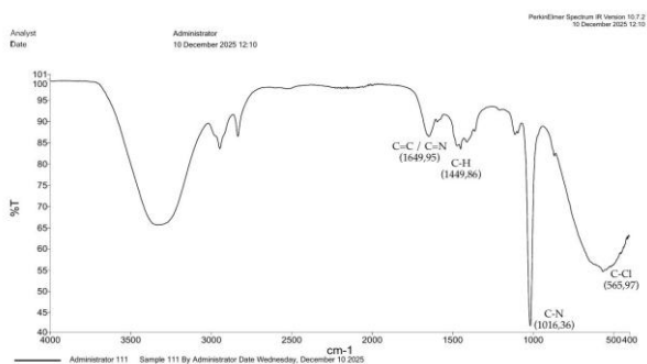
Gambar 3. Spektrum FTIR Standar CTM
