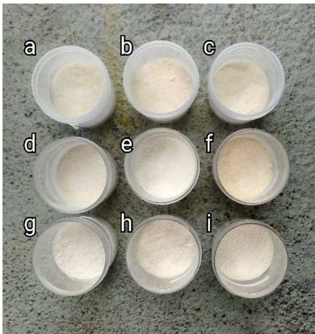
FIGURE 3. Hydroxyapatite synthesis results at (a) 140°C; 16 hours, (b) 160°C; 16 hours, (c) 180°C; 16 hours, (d) 140°C; 20 hours, (e) 160°C; 20 hours, (f) 180°C; 20 hours, (g) 140°C; 24 hours, (h) 160°C; 24 hours, and (i) 180°C; 24 hours.
