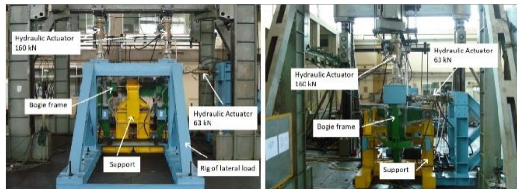
Figure 5. Monorail frame bogie prototype static test setup
