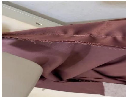
Figure 2 Puckered Seam Uniform Clothing
