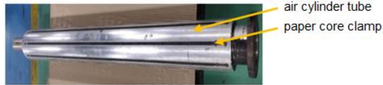
Figure 3. Air shaft type with air tube mechanism and single model paper core clamp
