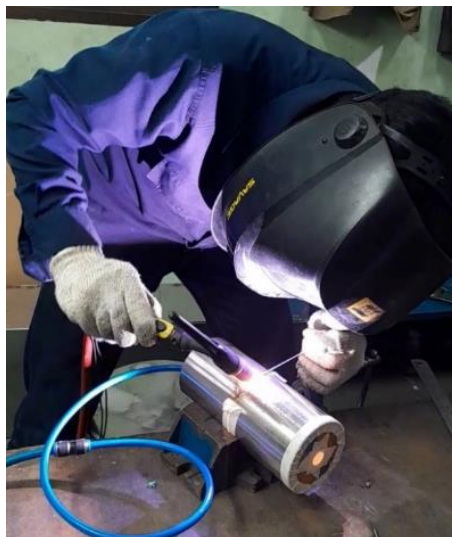
Gambar 6. Proses pengelasan GTAW specimen ASS 316L
