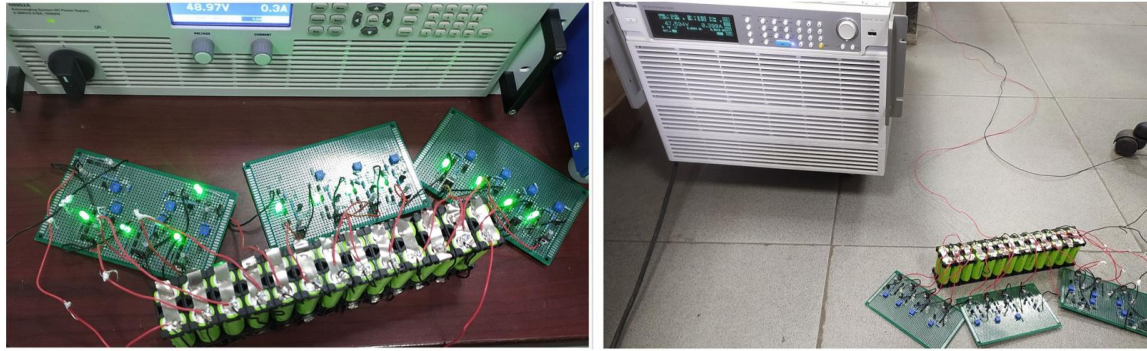
Figure 5: Hardware Charging and discharging through the proposed passive BMS
