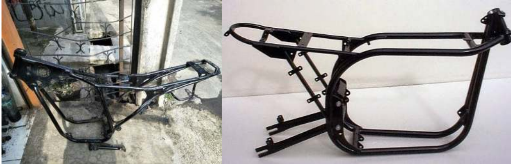
Figure 3 . Factory chassis (left) and custom chassis (right)
