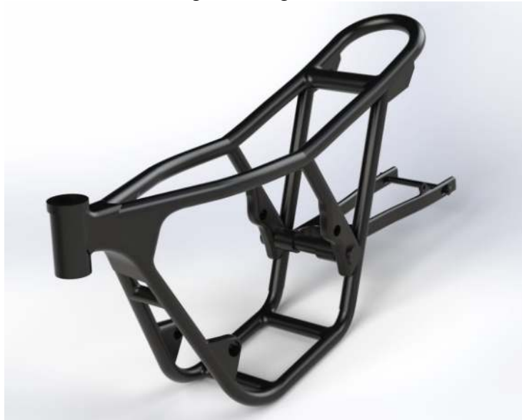
Figure 2. Two-wheeled motorcycle chassis design.
