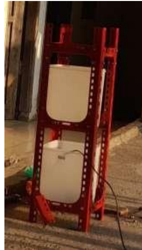
Figure. 5. Prototype of water control and monitoring at UG. PATIH drinking water depot
