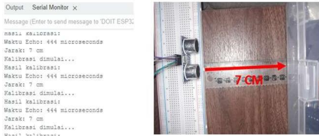
Figure. 8. Ultrasonic sensor testing
