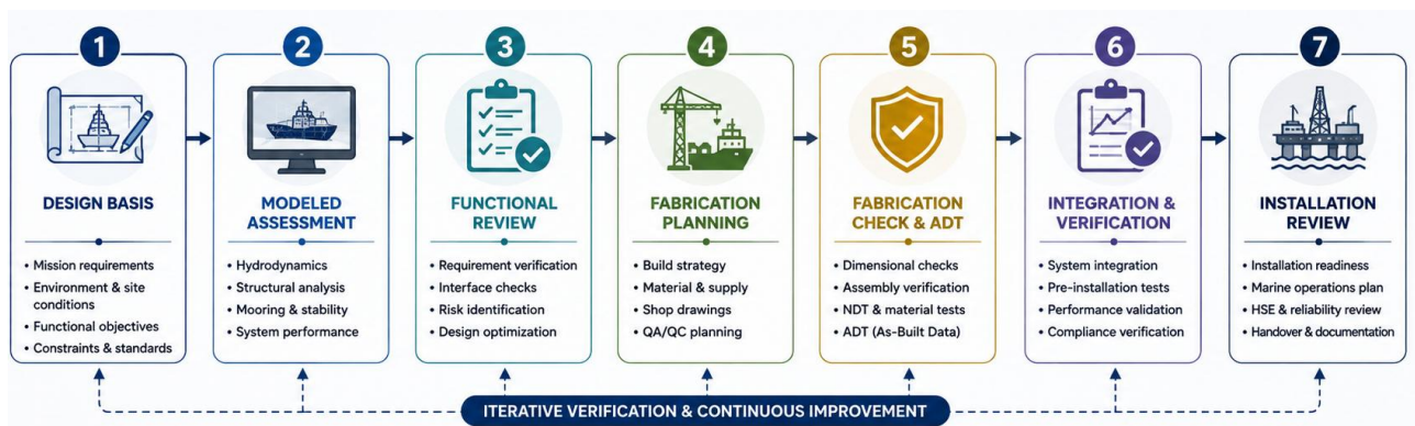
Figure 2. Integrated design–fabrication methodology adopted in this study.
