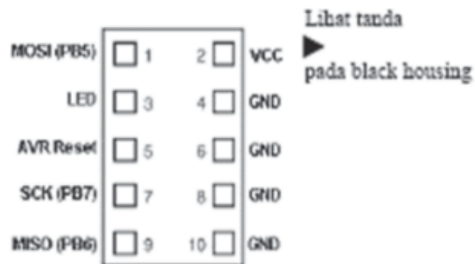
Gambar 5. Tata Letak Pin Black Housing de KITS AVR ISP Programmer Cable ( Prasimax Mikron Technology Development Center : 2007 )
