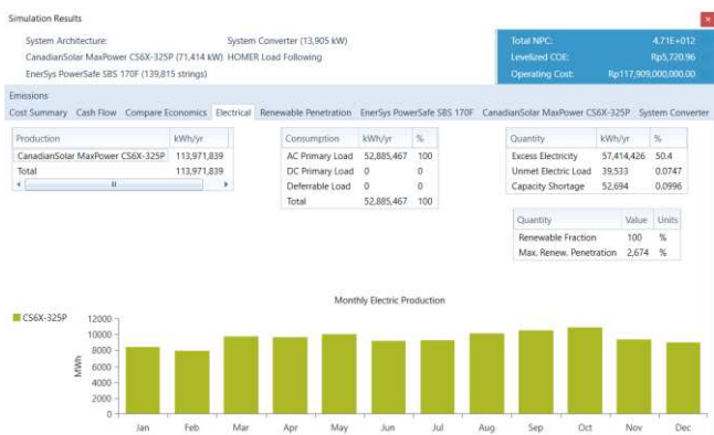
Figure 14. Simulation Result Operation PLTS-BESS
