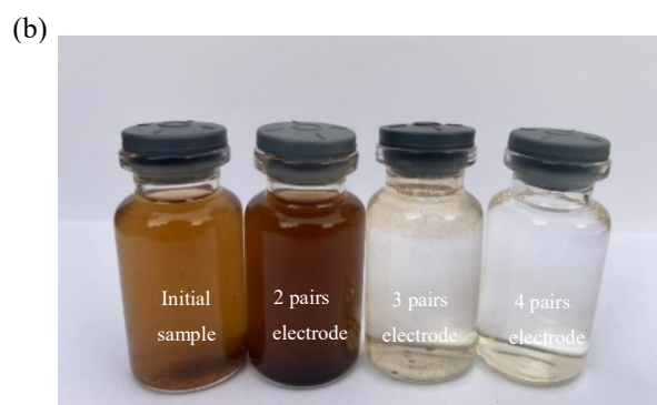
Fig. 4. (a) Effectiveness of electrode number to reduce the studied parameters and (b) the samples before and after treatment
