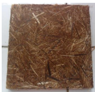
Figure 2. Composite board from sisal fiber and epoxy
