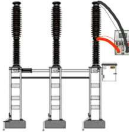
Figure 3. Contact Resistance Measurement Using DV Power
