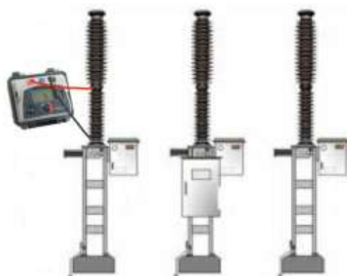
Figure 4. Insulation Resistance Measurement Using DV Power
