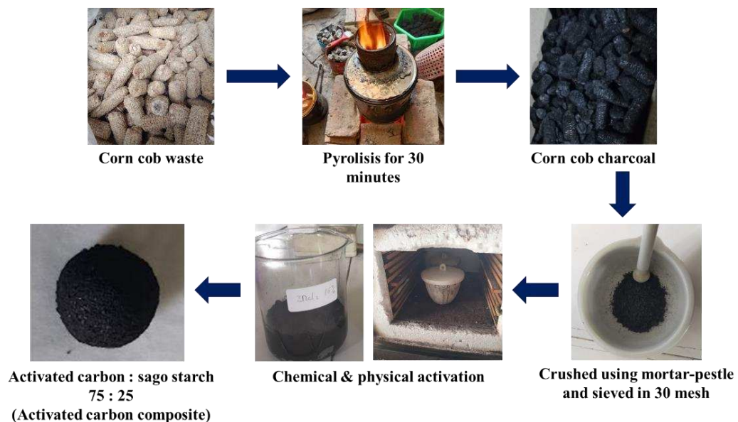
Figure 1. Corn cob activated carbon composite fabrication process
