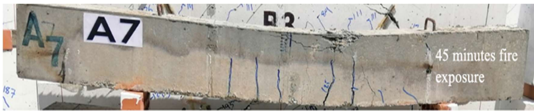
a) Experimental A7 beam cracking pattern
