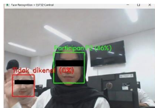
Fig. 8. Participant P2 Multi-Face Frame: The Enrolled Face Is Recognized (Confidence: 46%) While the Additional Face Is Rejected as Unknown (0%).
