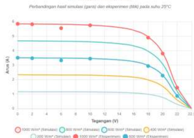
Figure 5. Characteristic curve of solar panels at various irradiancies
