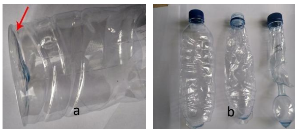
Gambar 11. Rough Parting Line (Tasnim, 2017)
