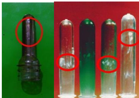
Gambar 4. Black Speckspadapreformbotol (Febryani, 2016)
