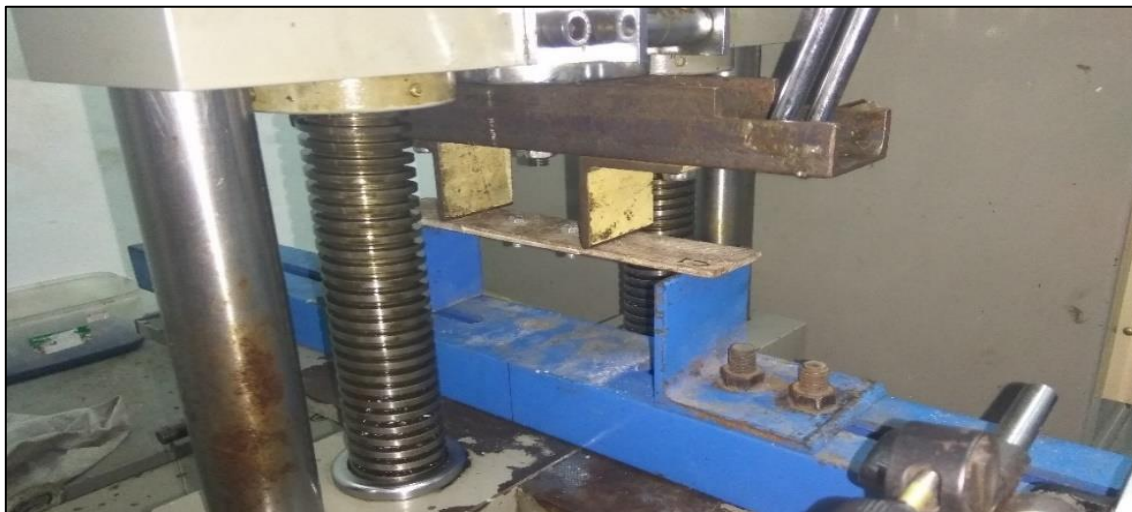
Figure 3. Flexural test configuration
