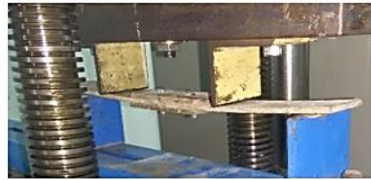
Stage 2 : Initial failure of matrix cracking
