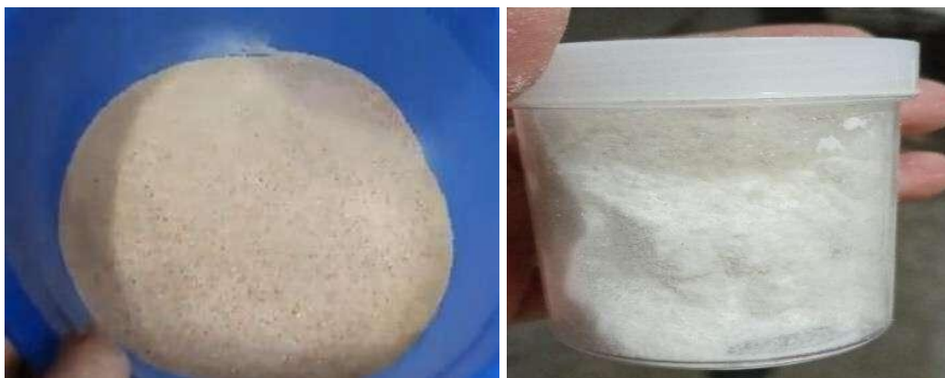
Figure 3. Appearance of chitosan from mangrove crab shells (left) and chitosan from vannamei shrimp shells (right)
