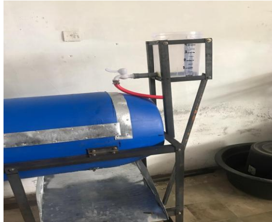
Figure 2. Bio-composter equipped with a microbial culture chamber
